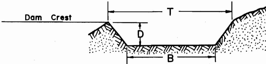
The bottom width of the spillway, B, will be 10" pipe..... feet.
