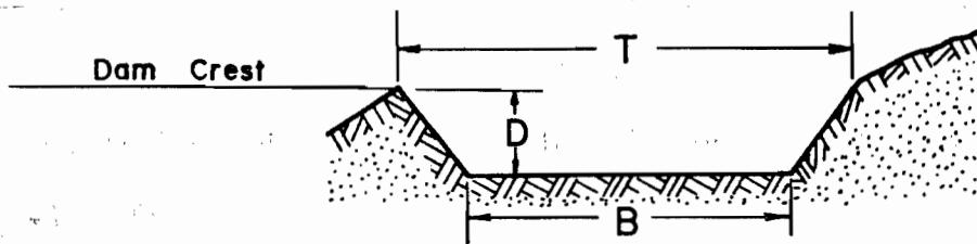
The bottom width of the spillway, B, will be .....14 16 feet.
