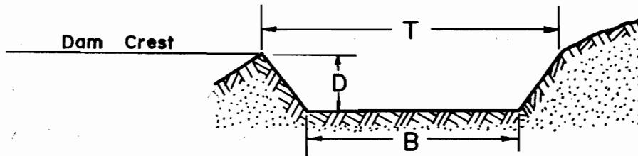
The bottom width of the spillway, B, will be .....TWO..... feet.
