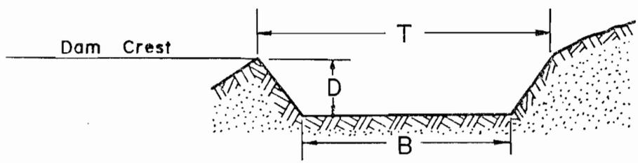
The bottom width of the spillway, B, will be ..... feet.
