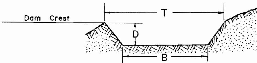
The bottom width of the spillway, B, will be .....3..... feet.
