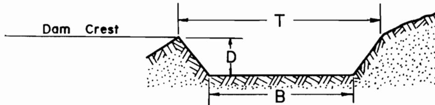
The bottom width of the spillway,  $B$ , will be 24 feet.
