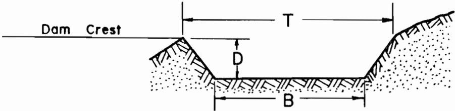
The bottom width of the spillway, B, will be 40 feet.
