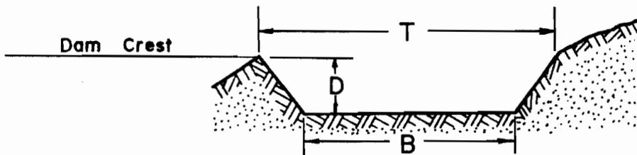
The bottom width of the spillway, B, will be 8.0 feet.
