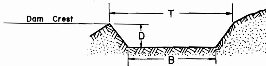
The bottom width of the spillway, B, will be .... Four feet.
