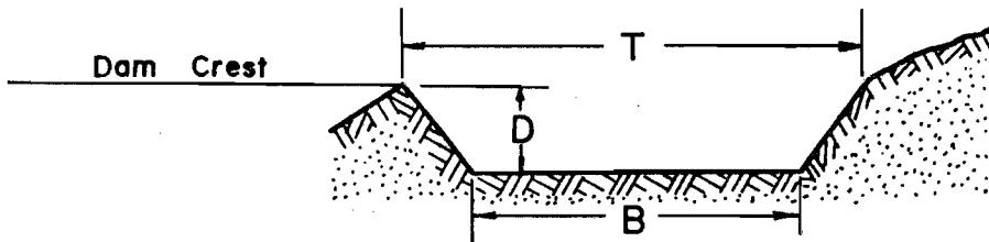
The bottom width of the spillway, B, will be ..... 26 ..... feet.
