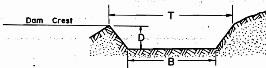
The bottom width of the spillway, B, will be ..... 2..... feet.
