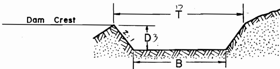
The bottom width of the spillway, B, will be 11.0 feet.
