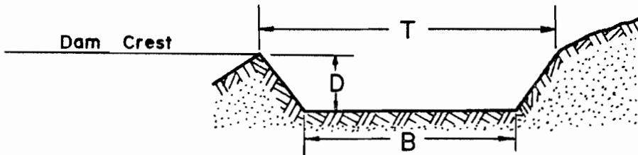
The bottom width of the spillway, B, will be ..... 200 feet.
