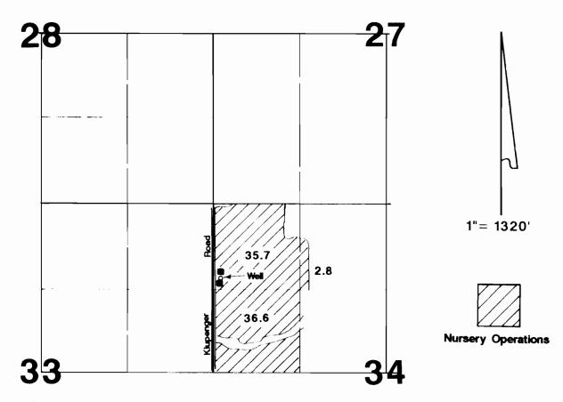
Well located 147'N & 132'E from NW corner SW1/4 NW1/4, Section 34.
