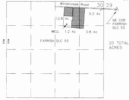
WELL IS LOCATED 1240 FEET SOUTH AND 2000 FEET WEST OF THE NORTHEAST CORNER OF SECTION 30
