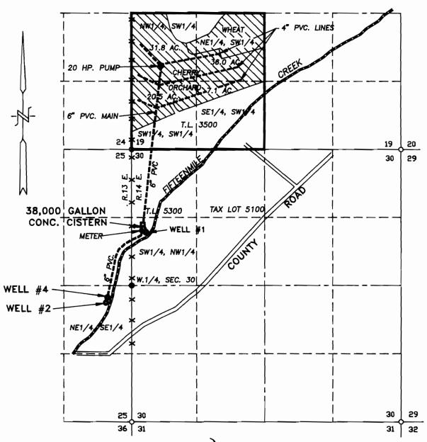
WELL #1 LOCATED 1030' N. & 280' E. WELL #2 LOCATED 330' S. & 500' W. ALL MEASUREMENTS ARE FROM THE W.1/4 CORNER OF SECTION 30. WELL #4 LOCATED 230' S. & 470' W. (E.I/4 CORNER, SECTION 25)
