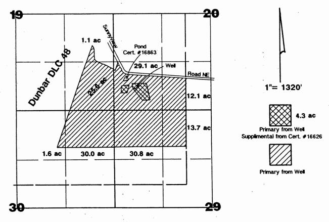
Well located 550'N & 580'E from SW cor. Section 20.
