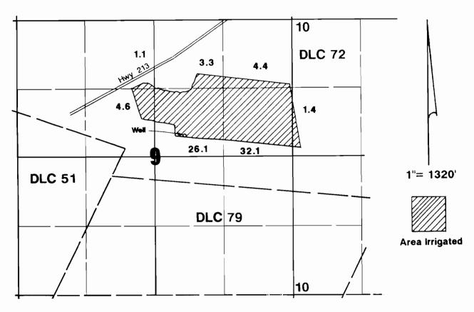
Well located 420'N & 580'E from center of Section 9.
