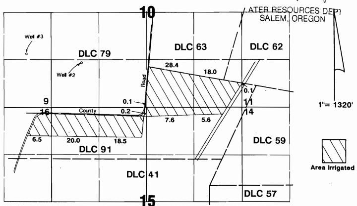
Well #2 located 1250'N & 850'E from the SW corner Section 10.
