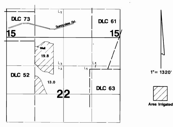
Well is located 1455'E & 440'S of NW corner Section 22.
