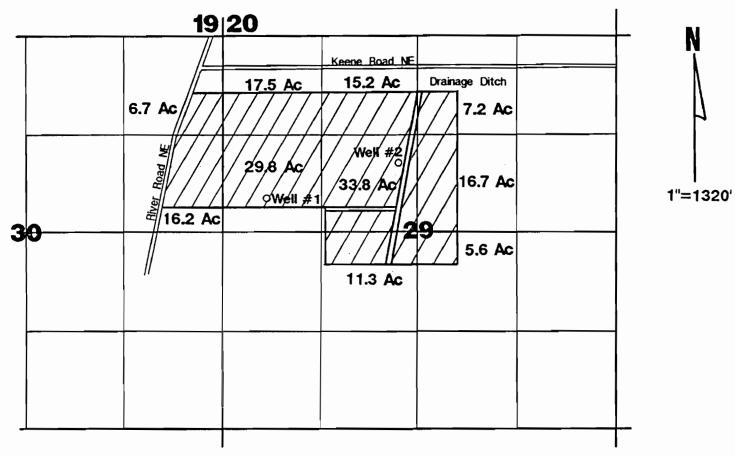
Well #1 located 2220'S & 600'E of NW Corner Section 29. Well #2 located 1725'S & 2390'E of NW Corner Section 29.
