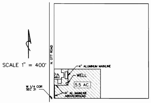
WELL LOC 210' N & 210' E OF W 1/4 CORNER OF SECTION 31.
