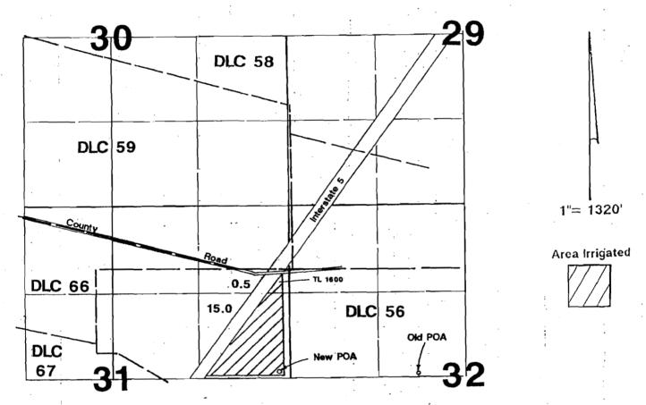
Old POA is located 60'N & 1950'E New POA is located 100'N & 150'W--both from the W1/4 corner of Section 32.
