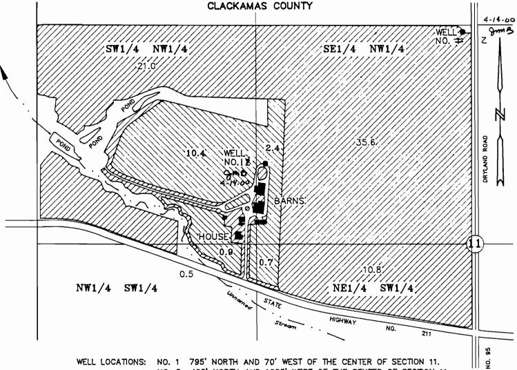
WELL LOCATIONS: NO. 1 795' NORTH AND 70' WEST OF THE CENTER OF SECTION 11. NO. 2 485' NORTH AND 1265' WEST OF THE CENTER OF SECTION 11.
