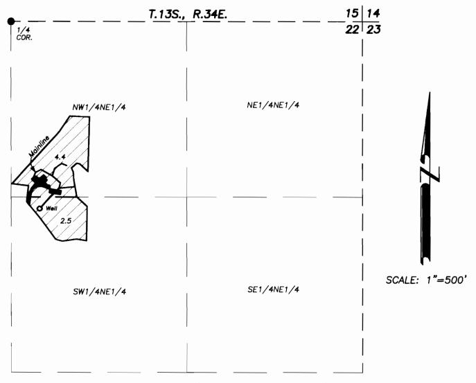
WELL AND POINT OF APPROPRIATION IS 1410'S. AND 210'E. OF THE N1/4 COR. SEC. 22, T.13S., R.34E.
