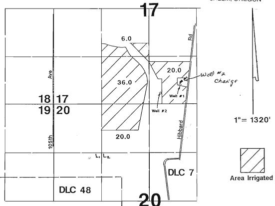
Well #1 located 550'N & 950'E from S¼ corner Section 17. Well #2 located 330'N & 300'E from S¼ corner Section 17.
