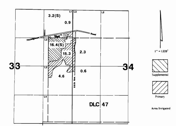
Well is located 1160'S & 520'W from the NE corner of Section 33.
