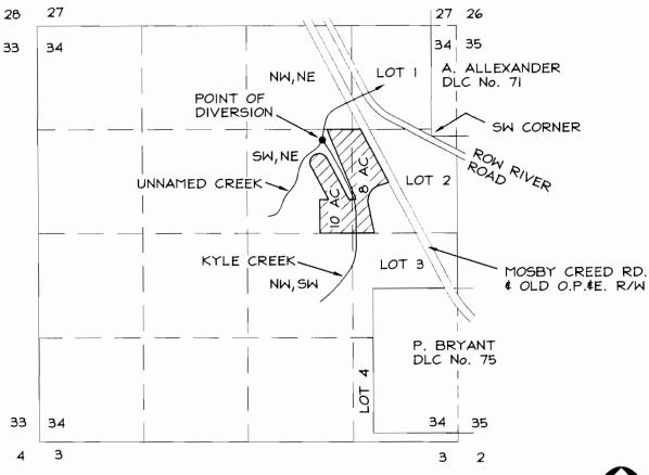
POINT OF DIVERSION IS LOCATED 48' SOUTH AND 1325' WEST OF THE SW CORNER OF DLC No. 71
