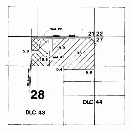
Well #1 is located 660'S & 350'E from the N1/4 corner of Section 28. Well #2 is located 462'S & 462'E from the N1/4 corner of Section 28.
