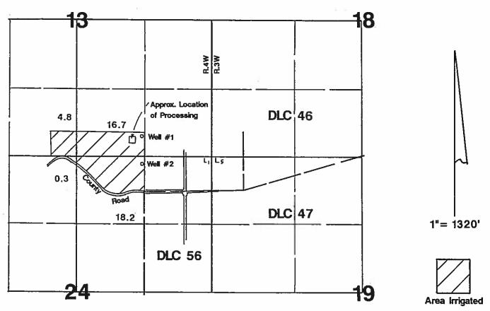
Well #1 located 1100'N & 50'W from NW corner DLC 56. Well #2 located 550'N & 50' W from NW corner DLC 56.
