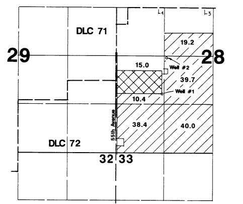
Well #1 located 1650'N & 1250'E from SW corner Section 28. Well #2 located 50'S & 1400'E from W1/4 corner Section 28.
