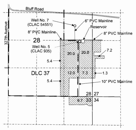
Well 5 (CLAC 00935) is located 2,600 feet north and 580 feet west of the SE corner of Section 28. Well 7 (CLAC 54551) is located 3,350 feet north and 820 feet west of the SE corner of Section 28.
