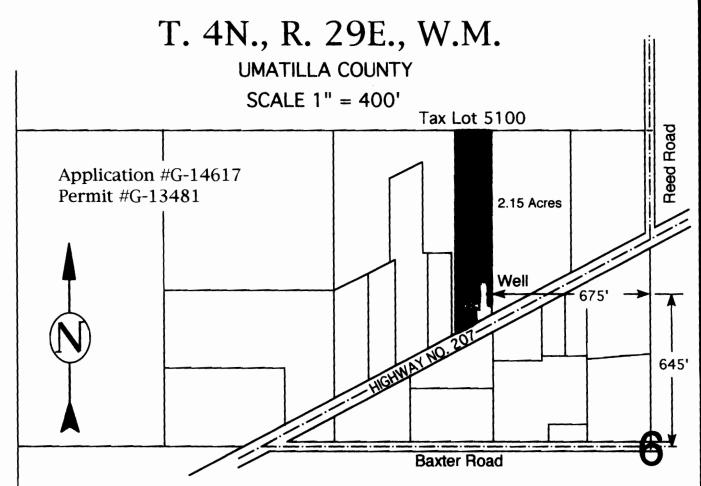
Well Located 645 Ft. North and 675 Ft. West of the Center Quarter Corner of Section 6, Township 4 North, Range 29 East, W.M., SE 1/4 of the NW 1/4 WGS84 - N 45° 51' 30.089", W 119° 14' 19.690"
