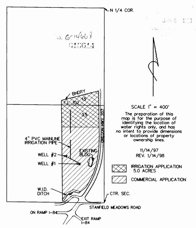
WELL #1 LOCATED 520' N & 330' W FROM CENTER SECTION 33. WELL #2 LOCATED 630' N & 510' W OF CENTER SECTION 33.
