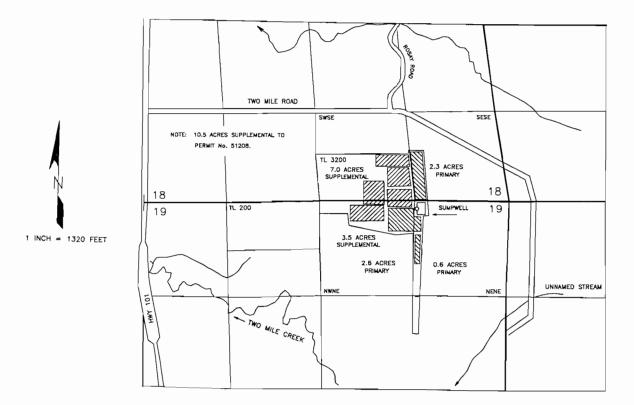
THE SUMPWELL POINT OF DIVERSION IS TO BE LOCATED 105 FEET SOUTH AND 1,265 FEET WEST FROM THE NORTHEAST CORNER OF SECTION 19 BEING WITHIN THE NE½NE½ OF SECTION 19, TOWNSHIP 29 SOUTH, RANGE 14 WEST, W.M., COOS COUNTY.
