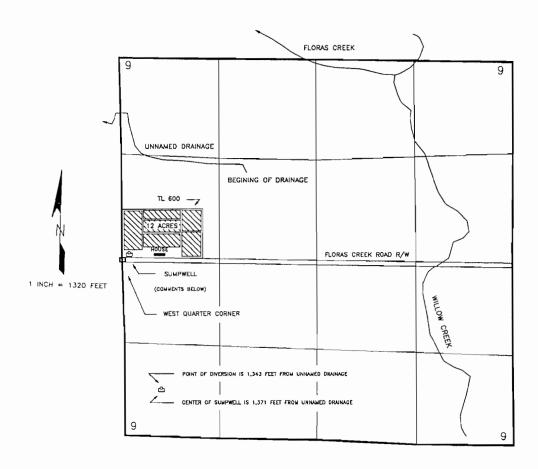
THE CENTER OF THE SUMPWELL IS TO BE LOCATED 70 FEET NORTH AND 85 FEET EAST FROM THE WEST QUARTER CORNER OF SECTION 9, BEING WITHIN THE SW¼NW¼ OF SECTION 9, TOWNSHIP 31 SOUTH, RANGE 15 WEST, W.M., IN CURRY COUNTY.
