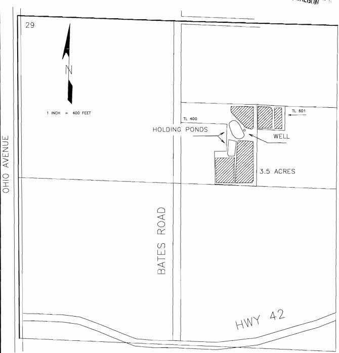
THE WELL IS TO BE LOCATED 960 FEET SOUTH AND 1,870 FEET EAST FROM THE NORTHWEST CORNER OF SECTION 29 BEING WITHIN THE NE'4NW'4 OF SECTION 29, TOWNSHIP 29 SOUTH, RANGE 14 WEST, W.M., COOS COUNTY.
