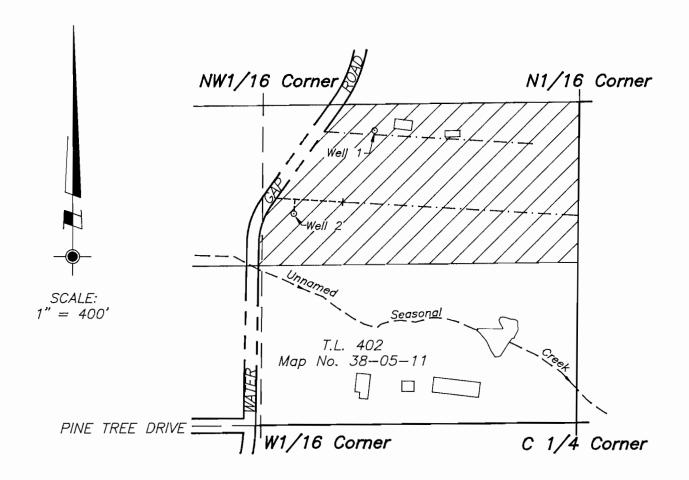
LEGEND: ----- Existing 2 1/2" PVC Pipe ---- Proposed 2 1/2" PVC Pipe Existing Buildings (Approximate Location) Proposed Place of use 18.4 Acres from Well 2 with any deficiency
