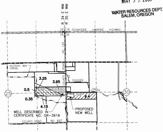
PROPOSED NEW POINT OF APPROPRIATION LOCATED 2890' SOUTH AND 200' EAST FROM THE NW CORNER OF SECTION 30
