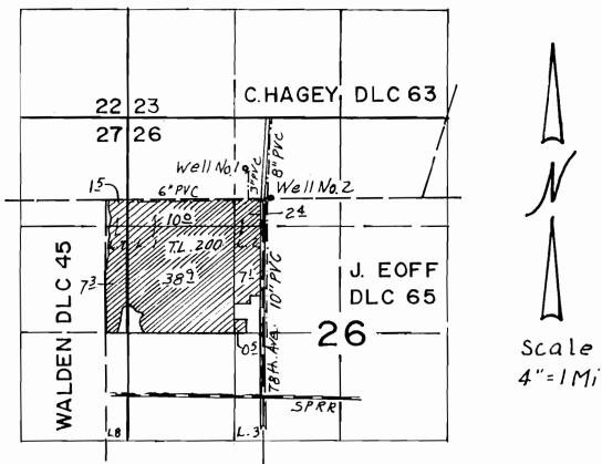
Well No. 1 Loc. 336'N & 200'W From NW COR. DLC 65 Well No. 2 Loc. 58' E from NW COR. DLC 65
