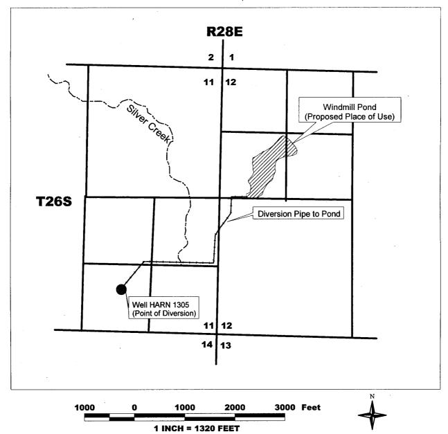
Point of Diversion, well HARN 1305, is located 850 feet north, 1930 feet west of the southeast corner of section 11, T26S, R28E, W.M.
