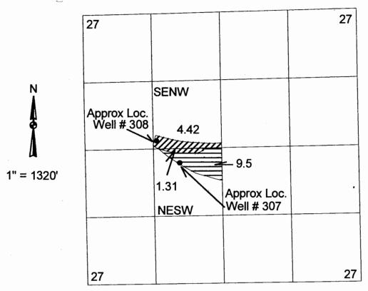
Well # 308 is approx 1400' E and 2470' S of NW corner of Sec 27 T13S R29E WM Well # 307 is approx 1840' E and 2915' S of NW corner of Sec. 27 T13S R29E WM
