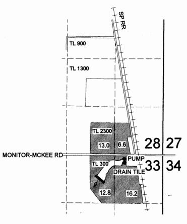
Drain Tile Div. Pt.: 190' south and 1595' east of the north 1/4 corner section 33
