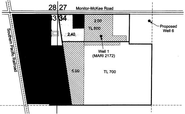
Well 1 (MARI 2172) is located 340 feet south and 610 feet east from the NW corner of Section 34. Well 2 (MARI 54098) is located 762 feet south and 32 feet east from the NW corner of Section 34. Proposed well 4 is located 910 feet south and 460 feet west from the NW corner of Section 34. Proposed Well 5 is located 340 feet south and 100 feet west from the NW corner of Section 34. Proposed Well 6 is located 120 feet south and 1,280 feet east from the NW corner of Section 34.
