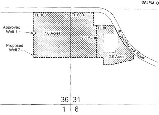
Approved Well 1 is located 1,000 feet north and 510 feet west from the SE corner of Section 36. Proposed Well 2 is located 700 feet north and 510 feet west from the SE corner of Section 36.
