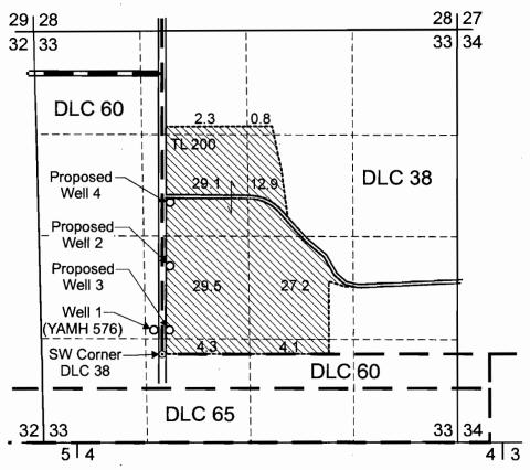
Well 1 (YAMH 576) is located 300 feet north and 90 feet west from the SW corner of DLC 38. Proposed Well 2 is located 1,100 feet north and 90 feet east from the SW corner of DLC 38. Proposed Well 3 is located 300 feet north and 90 feet east from the SW corner of DLC 38. Proposed Well 4 is located 1,900 feet north and 90 feet east from the SW corner of DLC 38.
