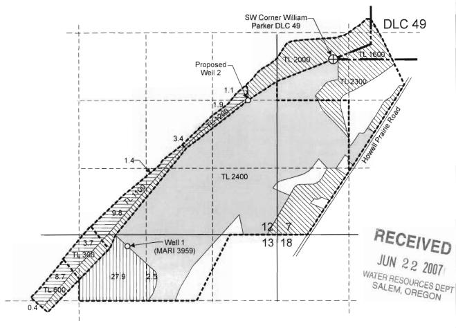
Existing Well 1 (MARI 3959) is located 210 feet south and 2,980 feet west from the NE corner, Section 13.
