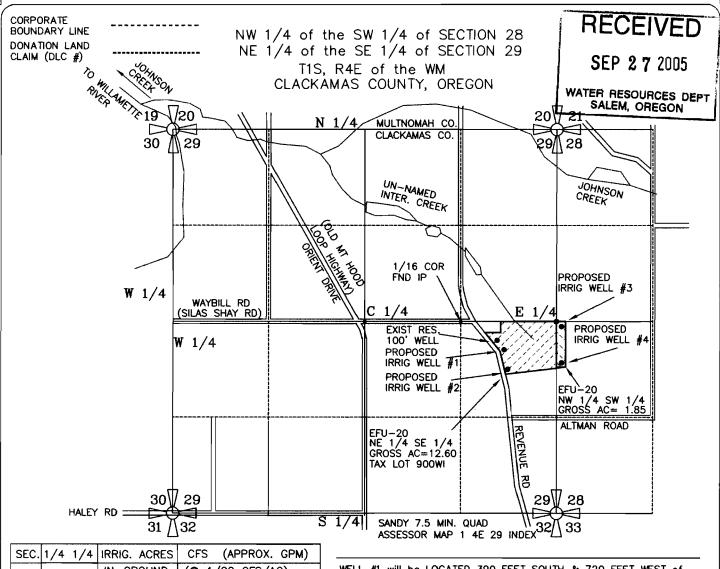
(@ 1/80 CFS/AC) 0.0225 CFS (10 GPM) IN-GROUND NW SW 1.80 ACRES 28 (@ 1/80 CFS/AC) 0.0700 CFS (31 GPM) IN-GROUND 5.60 ACRES NW SE 29 (@1/40 CFS/AC) 0.1500 CFS (67 GPM) ABOVE GRD NW SE 29 6.00 ACRES TOTAL 13.40 ACRES 0.2425 CFS (109 GPM)
