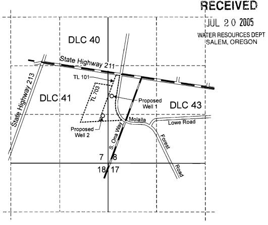
Proposed Well 1 is located 1,820 feet north and 100 feet east from the SE corner of Section 7. Proposed Well 2 is located 1,280 feet north and 140 feet west from the SE corner of Section 7. ----- Tax lot boundary
