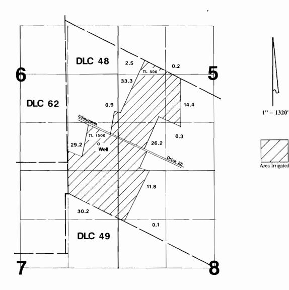
New well is located 750'N & 525'W from the SE corner of Section 6.
